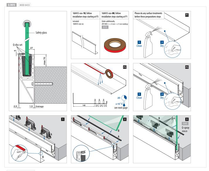
EASY GLASS® PRIME Y CLADDING - adhesive tape mounting instructions - Alternative mounting option
